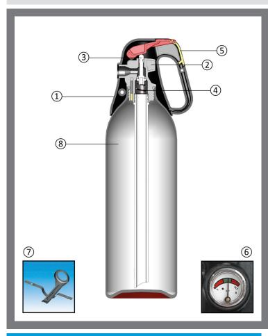
① The handy compact valve is ergonomically designed to guarantee an easy use with one hand. The construction material of the cap ensures a perfect protection against corrosion. The safety button – PUSH 1 – and the operating button PUSH 2 – are clearly visible.
